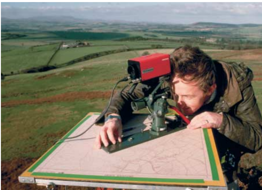
Figure 1 ► Cartographers in the field use technology to enhance the precision of their measurements. Electronic devices can be used to measure the distance between an observer and a distant point with a high degree of accuracy.
