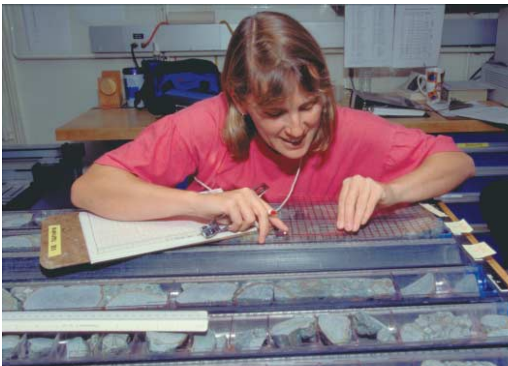
Figure 1 ► A scientist studies a core sample that was brought up from the drill aboard the research ship JOIDES Resolution .
