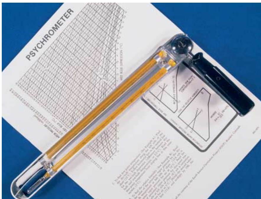
Figure 4 ► A psychrometer is commonly used with a table that lists relative humidity based on differences between wet-bulb and dry-bulb readings.
