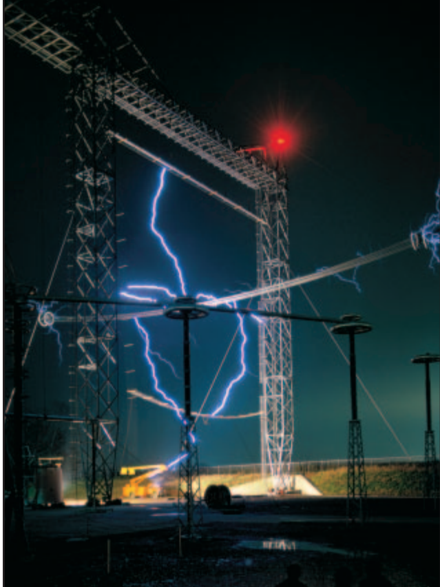
Figure 5 ► An outdoor ultrahigh-voltage laboratory generates artificial lightning to test its effects on electrical utility equipment. Research has led to the development of equipment that suffers less damage from lightning.
