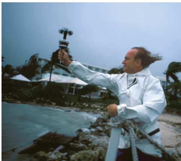
Figure 2 ► A meteorologist uses an anemometer during Hurricane Luis to measure wind speed.
