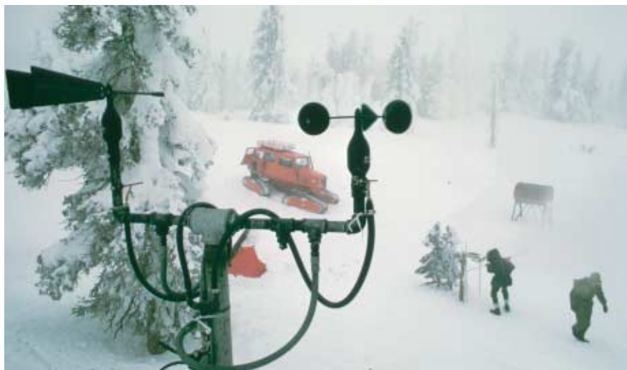
Figure 1 ▶ Weather instruments, such as these at Elk Mountain weather research facility in Wyoming, indicate wind speed and direction.
