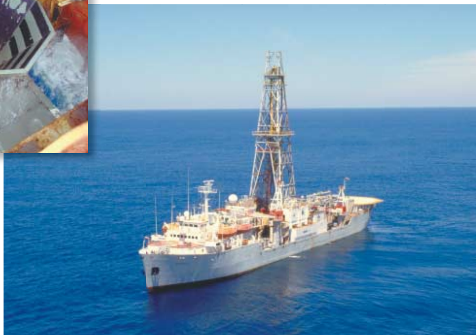
Figure 2 ► Reentry cones (above) are used so that core samples can later be taken from the same place on the ocean floor. Scientists aboard the research ship JOIDES Resolution (right) perform scientific studies of the ocean floor.
