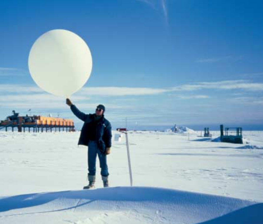
Figure 5 ► Scientists use weather balloons, such as this one in Antarctica, to send electric hygrometers into the high altitudes of the atmosphere.
